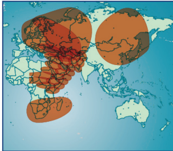
Gambar 15. Multispot beam Ka-band
